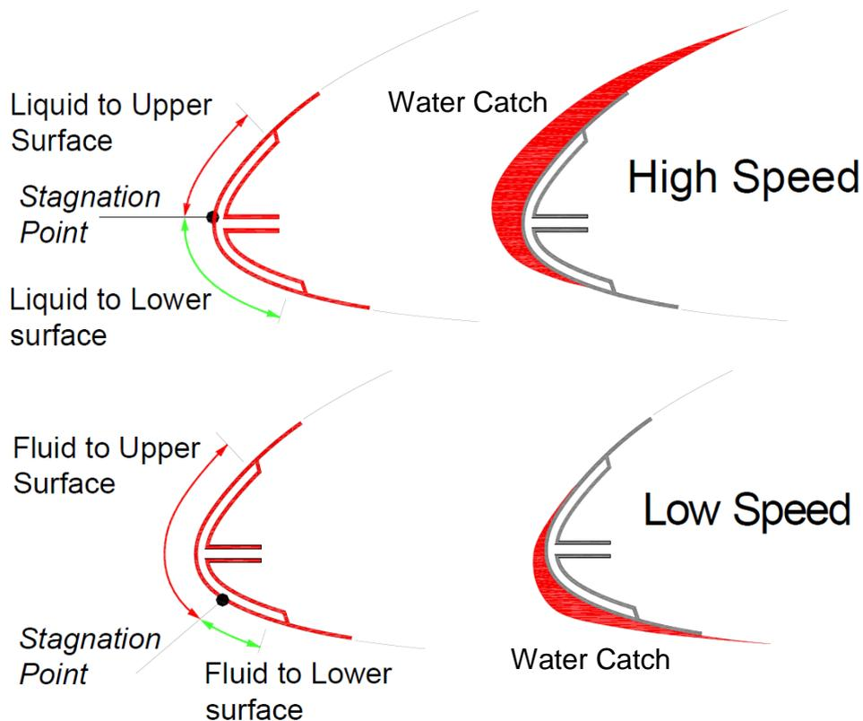
**Figure 7: Effects of Stagnation Point on Water and Fluid Distribution**
