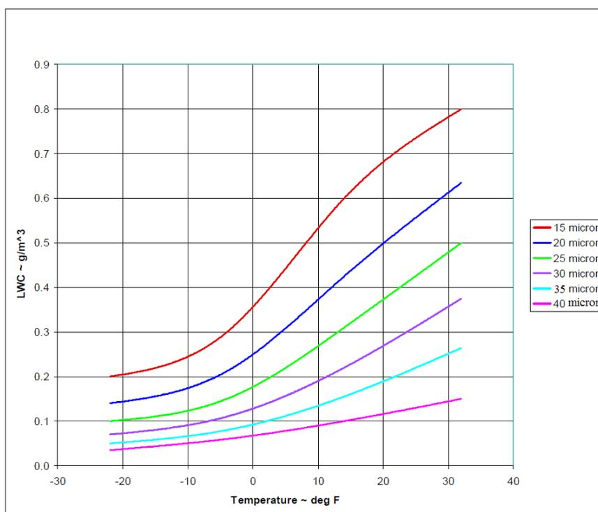
Figure 3: Continuous Maximum Icing Envelope as a Function of Temperature
