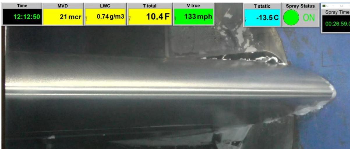
Figure 18: After ET Zone Activation (32.5 kW/m<sup>2</sup>)
