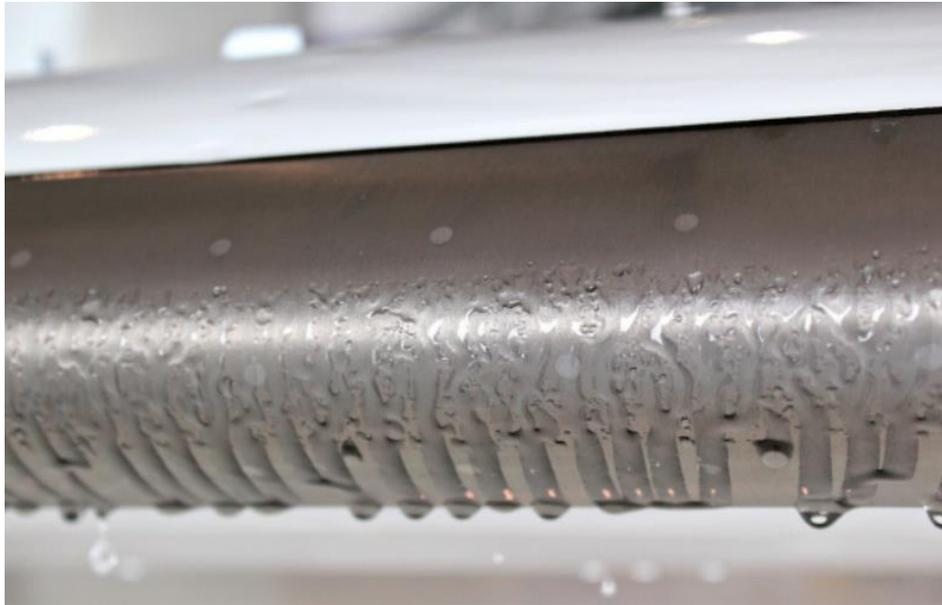
**Figure 1: FPD Fluid Flowing from a Porous Panel**
