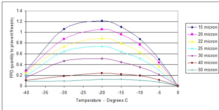
Figure 6: Intermittent Maximum Critical Temperature
