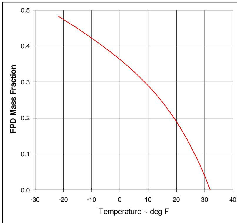
Figure 4: Ice Protection Fluid Mass Fraction Characteristics
