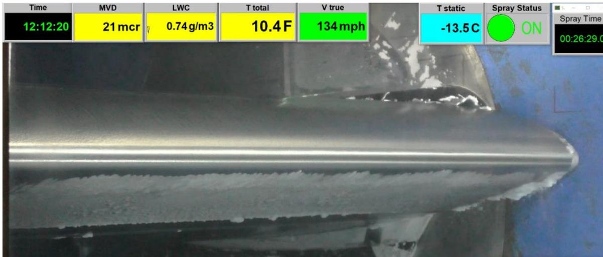
Figure 17: Parting Strip at 17.3 ml/min and Prior to ET Activation
