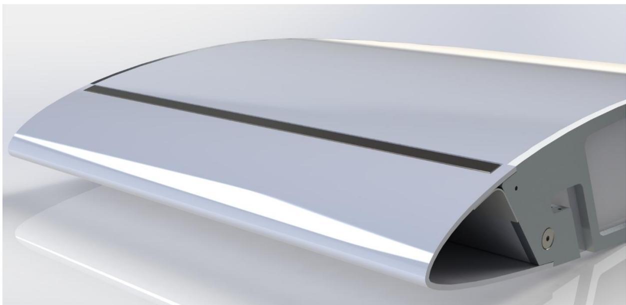
**Figure 12: Implementation of an FPD SLD/Runback Zone**
