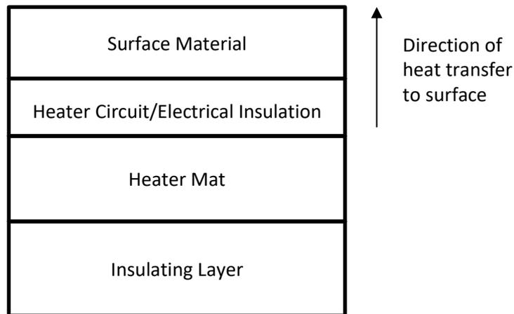
**Figure 9: Basic Construction of a Heater Mat on a Structural Substrate**
