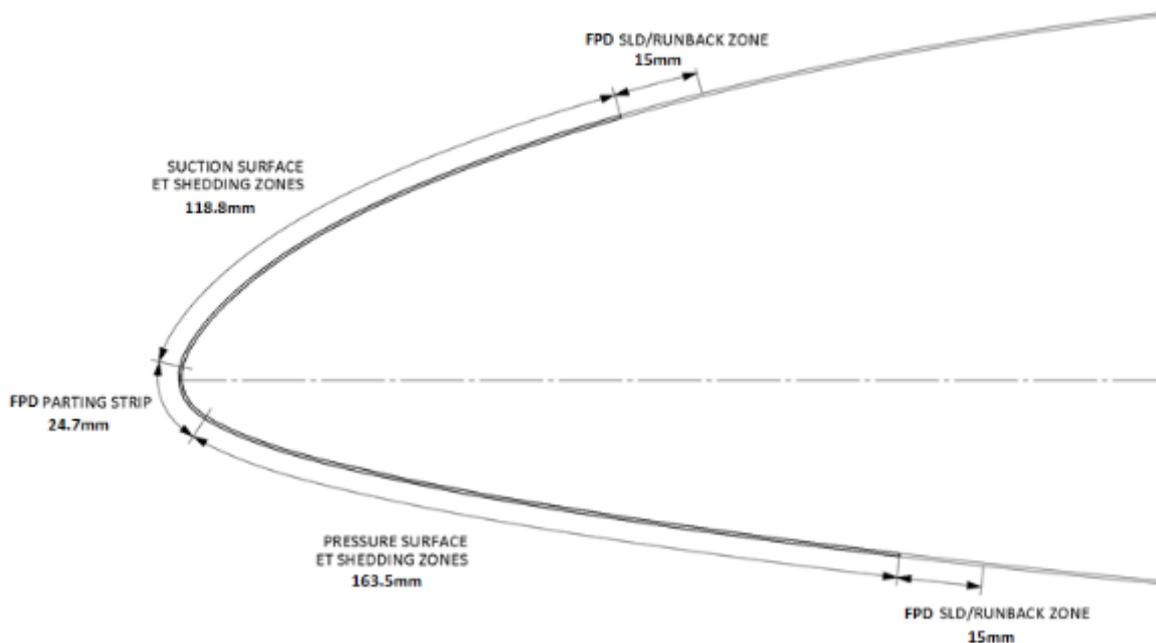
**Figure 14: Zones of the Hybrid Test Model**
