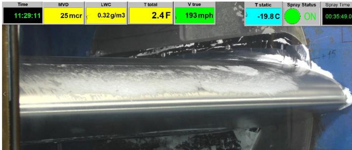
Figure 15: Parting Strip Optimized (16.8 ml/min) and Prior to ET Activation
