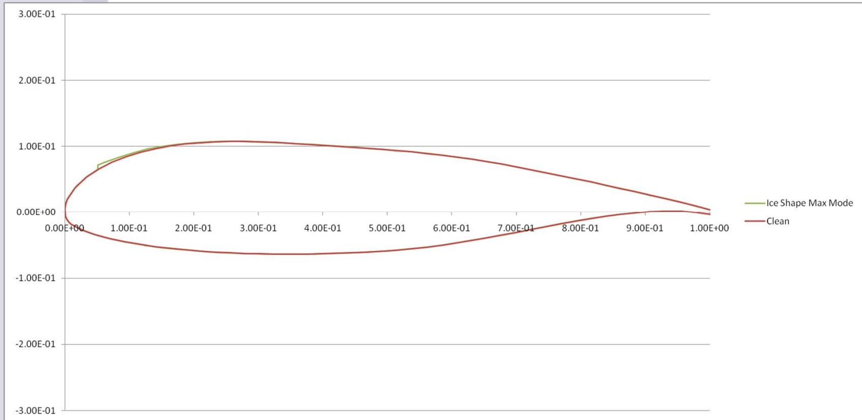
Wing at 110 m/s TAS at an AOA of -2.2 with a chord of 125 cm.
