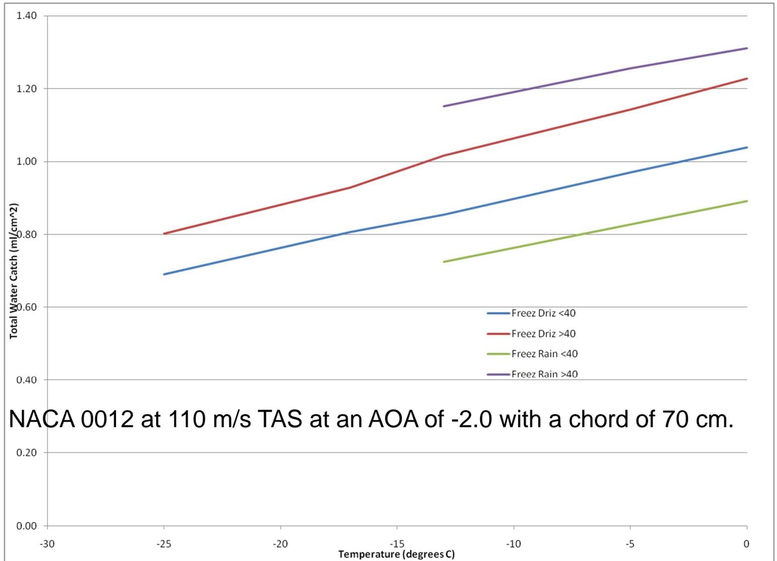
NACA 0012 at 110 m/s TAS at an AOA of -2.0 with a chord of 70 cm.
