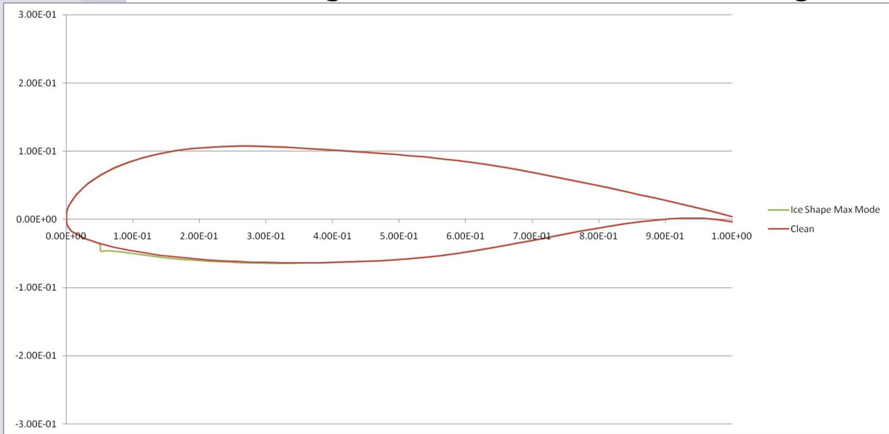
Wing at 75 m/s TAS at an AOA of 2.2 with a chord of 125 cm.
