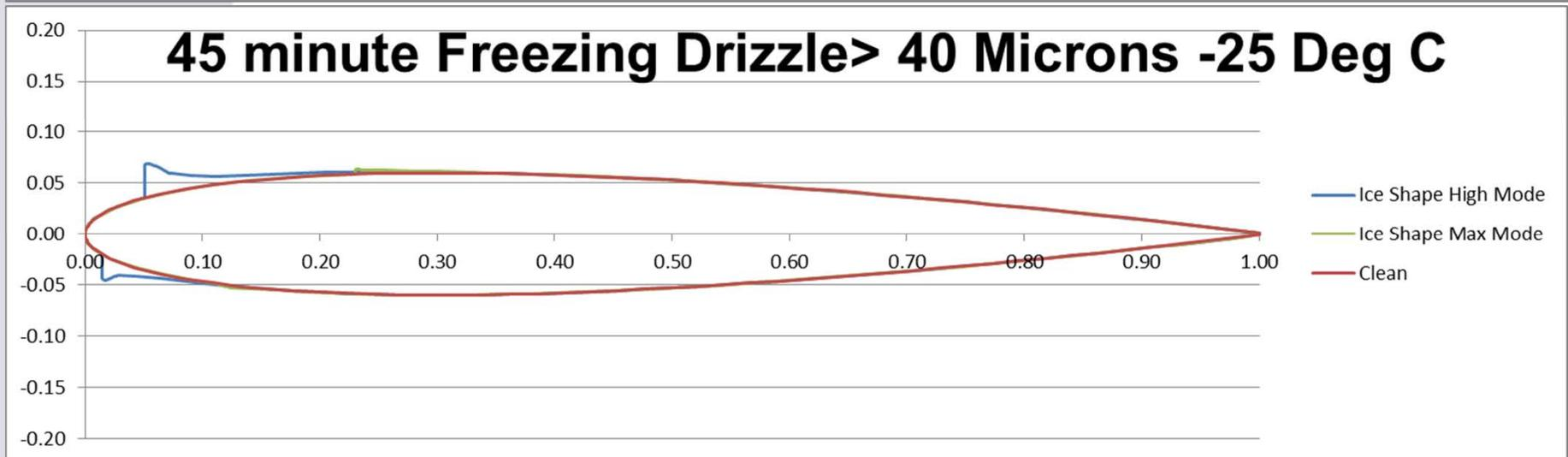
NACA 0012 at 110 m/s TAS at an AOA of -2.0 with a chord of 70 cm.
