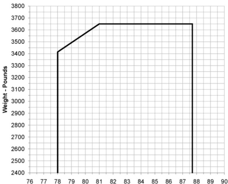
Figure 2-1 Bonanza G36 Center of Gravity Limits for Flight into Known Icing Conditions
