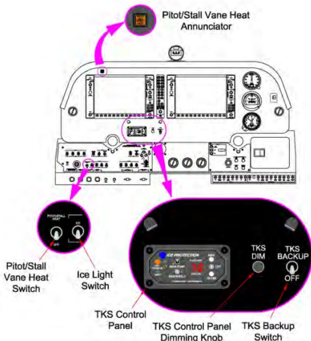
**Figure 8-3 Bonanza G36 Instrument Panel With TKS System Installed**
