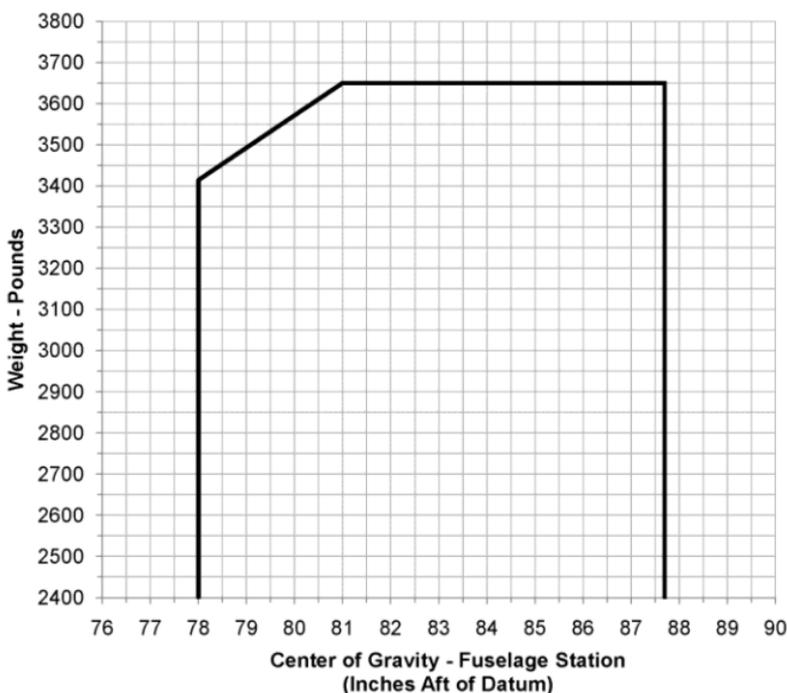
**Figure 6-1 Bonanza G36 Weight and Balance Limits for Flight into Known Icing Conditions**
