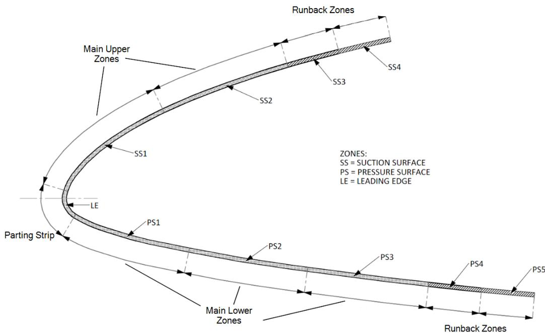
**Figure 10: Example of an Electrothermal Leading Edge**
