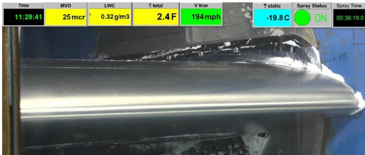
Figure 16: After Activation of the ET Zone (8 kW/m<sup>2</sup>)
