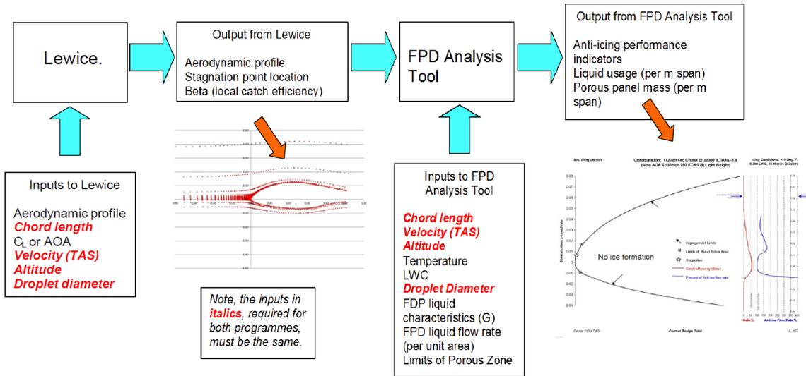
Figure 8: Typical Panel Design Workflow
