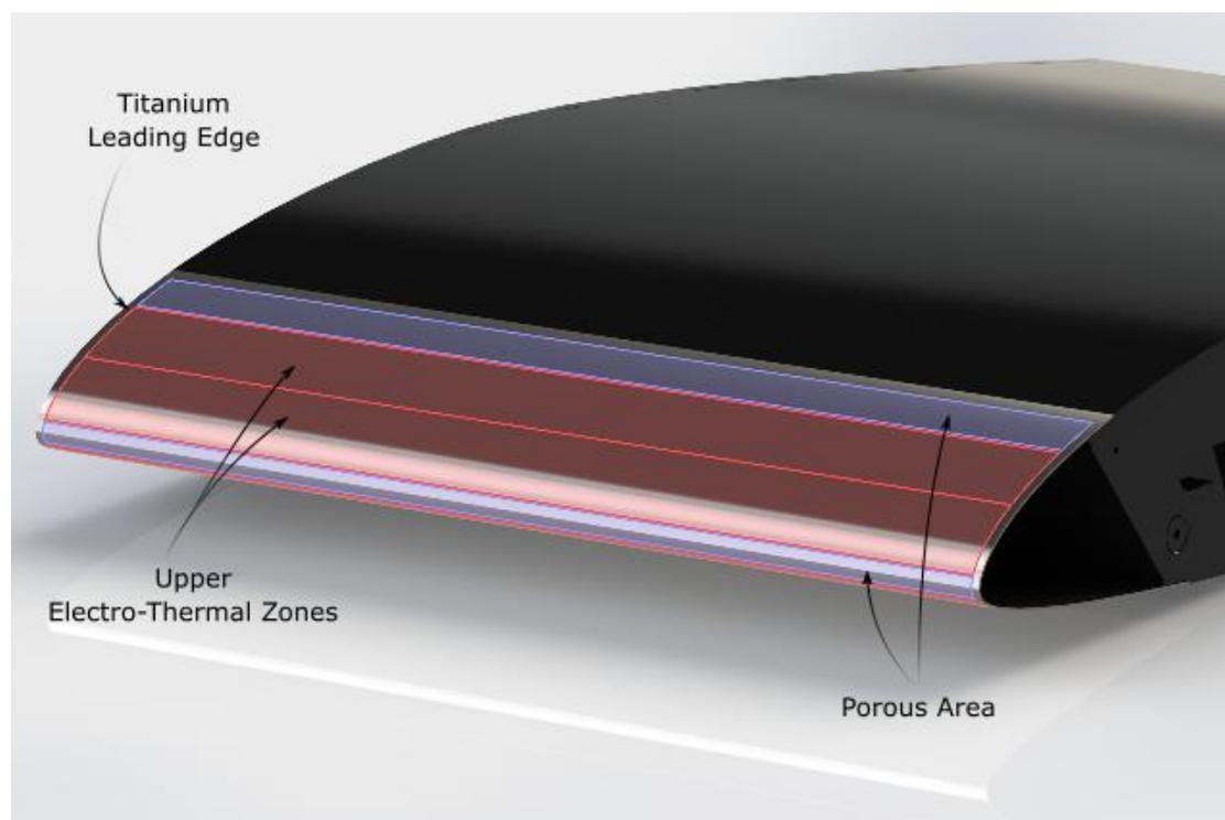
**Figure 11: Hybrid Leading Edge Layout (Bottom Zones not Shown)**
