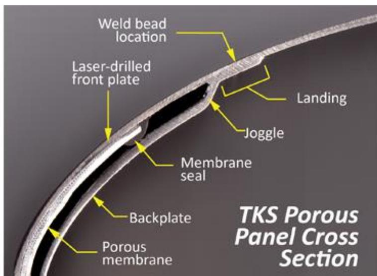
**Figure 2: Cross Section of a Typical Porous Panel**
