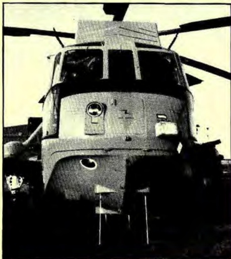
TKS strips are fitted to the deflector shields in front of the air intakes on many Sea Kings. They proved to be valuable assets in the frequent icing conditions of the Falklands conflict.
