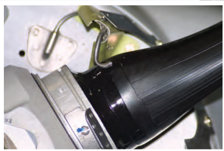
Propeller slinger ring installation on a PA-32. The slinger feed tube delivers fluid to the prop blade.
