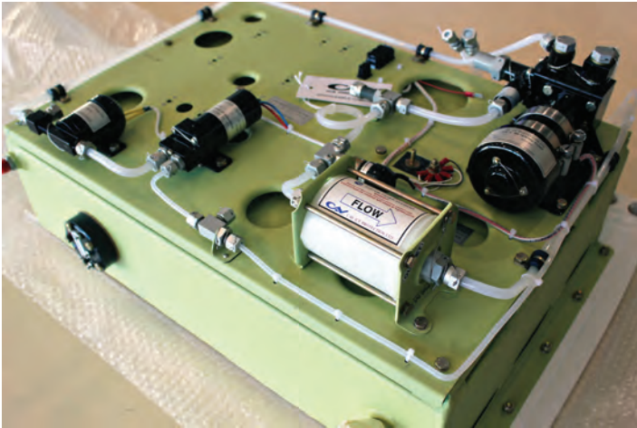
An uninstalled TKS equipment pallet for a Cessna 206. The light green box is the fluid tank.
