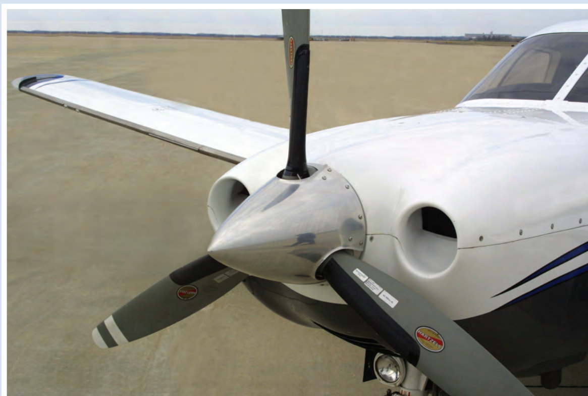
TKS installation on a PA-32 propeller.
