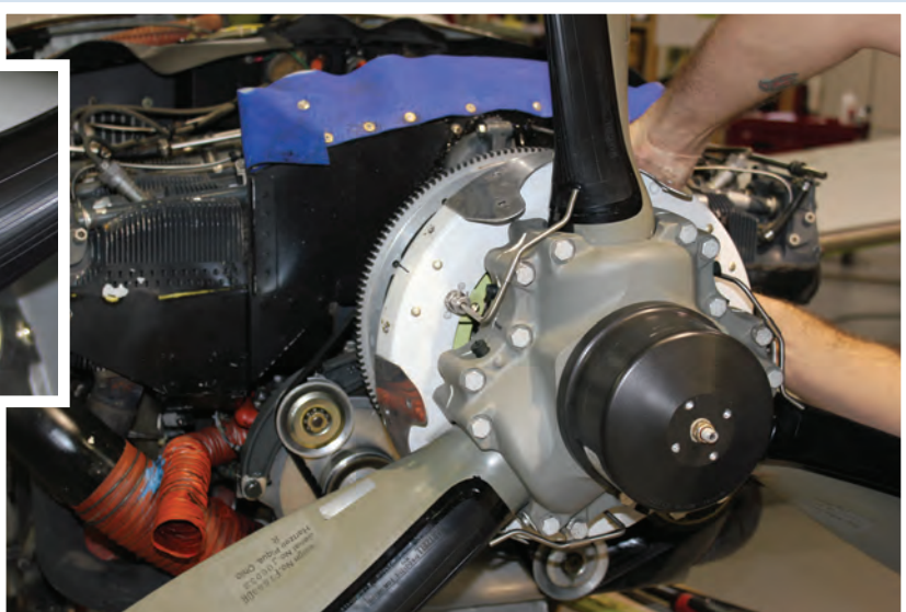
Propeller slinger ring installation on a PA-32. The slinger feed tube delivers fluid to the prop blade.
