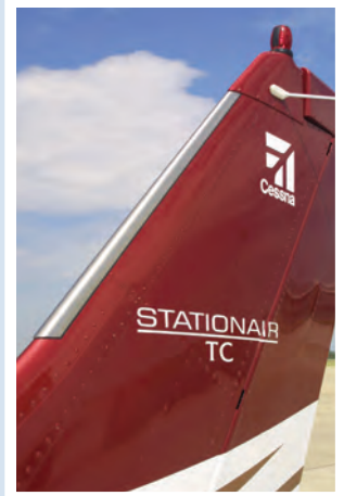
TKS panels are installed on the vertical and horizontal stabilizers of the Cessna 206.
